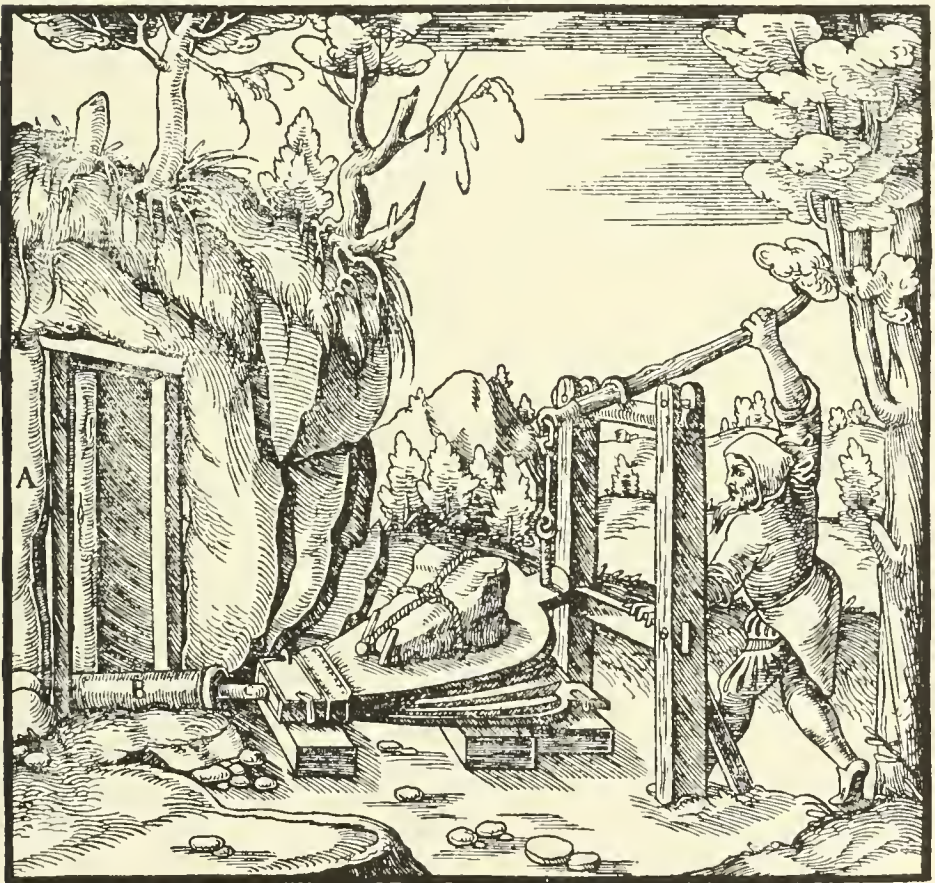
A—TUNNEL. B—PIPE. C—NOZZLE OF DOUBLE BELLOWS.
